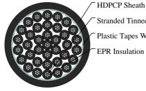
HDPCP Sheath Stranded Tinned Copper Conductor Plastic Tapes Wrapping EPR Insulation
